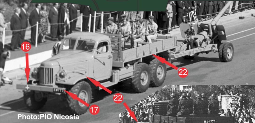
The ZIL 157 truck was used to tow the 100 mm Model 1944 gun. These were finished in sand until 1972 when the finish became dark green. The position of the various markings was the same for both colour schemes.
