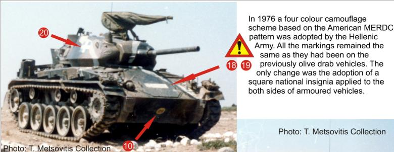
With the adoption of the four colour camouflage, M24 light tanks were repainted probably using the MERDC pattern for the M48 tank. This was adapted to the smaller tank in keeping with the principles of the scheme but the results were never standard.
